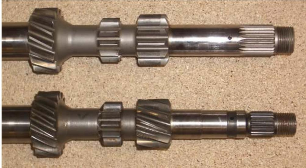
As you can see below, it is the step changes where the trouble starts. these are two broken 5th gear ends from two different gearboxes which have failed in a very similar way, starting at the undercut.
