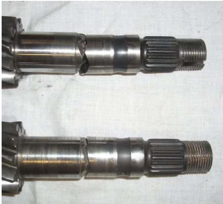
The EN 36 shaft has given no trouble, and has withstood full power and torque in all gears including 5<sup>th</sup> at the Nurburgring (185 mph and still going). Further kits have been used in GT 40 replicas actively used in sprinting and hill climbs, including some with tuned 351 Windsor's and the only thing they have broken is drive shafts!
