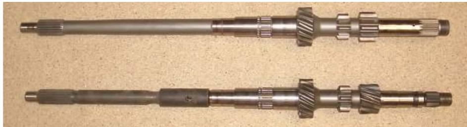
As you can see, the new shaft (upper shaft in photo above) eliminates the necking where the clutch and first motion shafts join, is larger in diameter wherever possible, and particularly so at the (overhung) 5th gear end which is substantially thicker, and has no undercut. the clutch spline is bigger as is first gear. You can see the 5th gear end in detail below. Note no stress raisers in the form of step changes in diameter or undercuts, and larger in diameter throughout.
